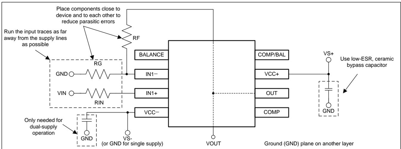
Figure 16. Operational Amplifier Board Layout for Noninverting Configuration
