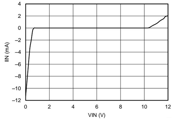
**Figure 13. Current Drawn by the Input of the Voltage Follower ( $I_{IN}$ ) vs the Input Voltage**
