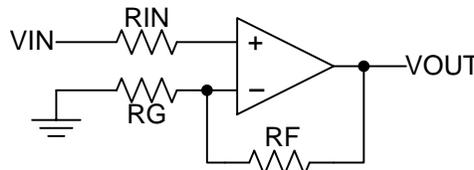
Figure 15. Operational Amplifier Schematic for Noninverting Configuration
